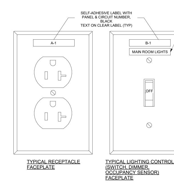
1 WIRING DEVICE LABELING DETAIL E001 NOT TO SCALE
