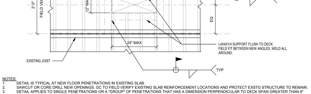
A GROUP OF PENETRATIONS FITTING WITHIN THE MAX DIMENSION INDICATED SHALL CONSTITUTE A SINGLE PENETRATION. PROVIDE MIN. 1.5" DECK BEARING AT NEW SUPPORT AN
